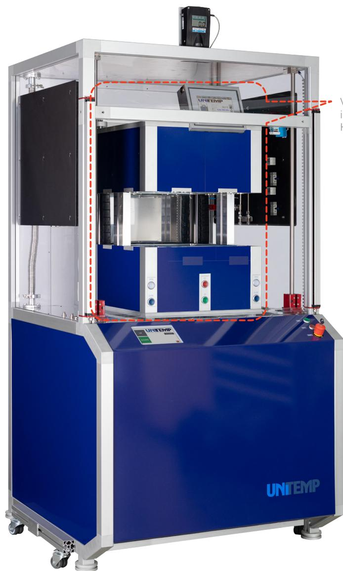
VPO-300 oven integrated in a Safety Hood for pure Hydrogen application
