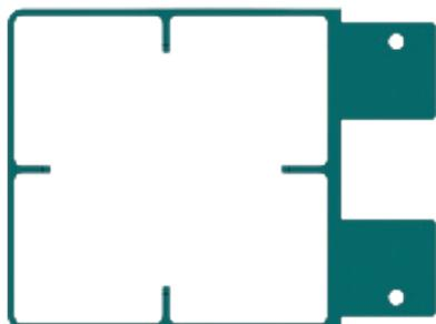
Standard Quartz holder for 100 mm wafer size
