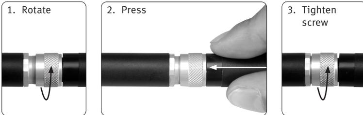
**!** Only a properly assembled and fixed connection assures the IP protection rating.
