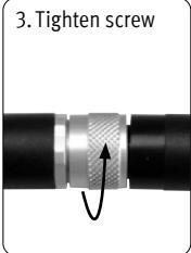
**!** Only a properly assembled and fixed connection assures the IP protection rating.
