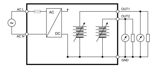
The maximum permissible cable length can be determined under consideration of the voltage drop on the cable.
