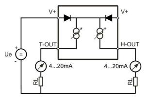
The maximum permissible cable length connecting the HF52 to other devices is determined by the total resistance resulting from the addition of the cable resistance and that of the devices connected in series with the unit.
