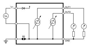
The maximum permissible cable length, connecting the unit to other devices, is determined by the total resistance resulting from the addition of the cable resistance and that of the devices connected in series with the unit.
