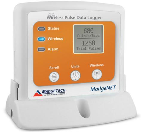
The RFPulse2000A is a wireless data logger that records pulse output signals from various sensors such as flow meters and anemometers. When started, the data logger samples at 100Hz and at the user specified reading rate, recording the total number of pulses from the sample to memory.
