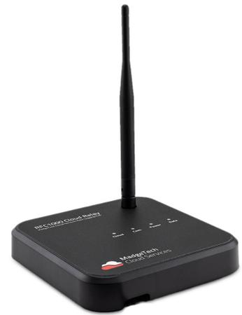
The RFC1000-CE Cloud Relay is a small, powerful device which transmits real-time and recorded data directly to the MadgeTech Cloud without the need of a central PC. With the RFC1000-CE Cloud Relay and MadgeTech Cloud Services, real-time data is easily viewed from any internet enabled device, anywhere in the world.
